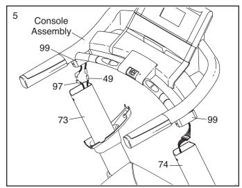
Partially tighten three 3/8" x 1 1/4" Bolts (64) with three 3/8" Star Washers (90) into the Right Upright (74). Next, partially tighten three 3/8" x 1 1/4" Bolts with three 3/8" Star Washers (not shown) into the Left Upright (73). Then, firmly tighten the six Bolts.
